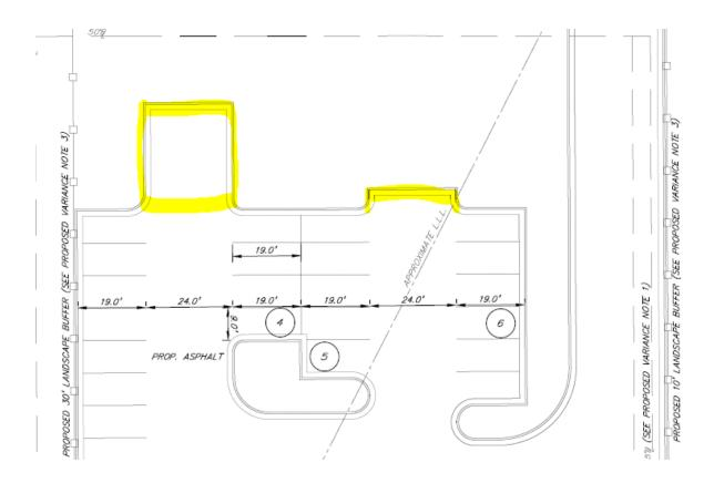
Attachment showing paving to be removed or where barriers to vehicle travel are to be installed.
